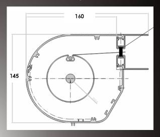
The SZ-MSW 1000 system with ZIP-system is always provided with SZ-MSW guides with measures of 65 mm. x 45 mm. Rectangular systems can be supplied with screen - or acrylic fabric.
